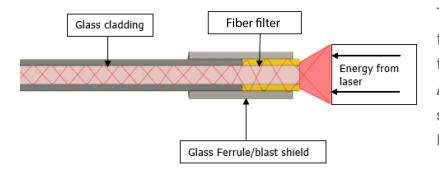
The Excalibur fiber inhibits stray energy from entering the cladding layer, preventing thermal damage to the fiber and ureteroscope. An additional glass ferrule serves as a blast shield, preventing energy from damaging the laser's optics.
